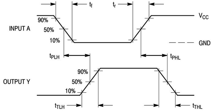
Figure 1. Switching Waveforms
