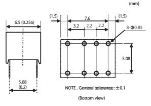
Tolerance of lead pitch is  $\pm 0.15$ mm (0.006inch) Other tolerances  $\pm 0.3$ mm (0.012inch)
