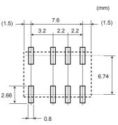
Tolerance of lead pitch is  $\pm 0.15$ mm (0.006inch) Other tolerances ±0.3mm (0.012inch)
