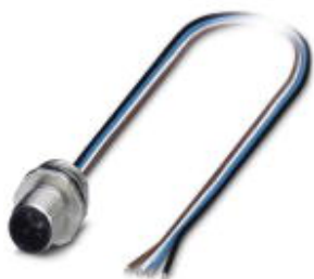
Sensor/Actuator flush-type plug, 4-pos., M12, A-coded, front/screw mounting with M16 thread, with 0.5 m TPE litz wire, 4 x 0.34 mm 2
