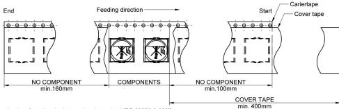
Packaging is referred to the international standard IEC 60286-3:2007 Projection -180° Würth Elektronik eiSos GmbH & Co. KG EMC & Inductive Solutions шшшш Max-Eyth-Str. 1 74638 Waldenburg Germany Pull-of force 2015-06-08 SSt PSL Tel. +49 (0) 79 42 945 - 0 12 mm 0,1 N - 1,3 N www.we-online.com Tape width SSt 1.0 2014-11-11 PSL 16 mm 0,1 N - 1,3 N
