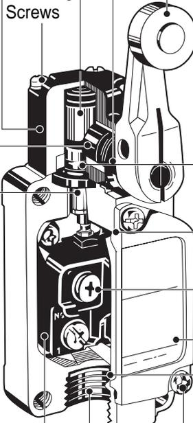
\* By changing the direction of the operational plunger, any one of the three operational directions (both sides, left, or right) can be selected.
