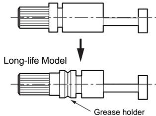
Smooth movement is achieved using olefin grease. (Standard models use molybdenum disulfide grease.)
