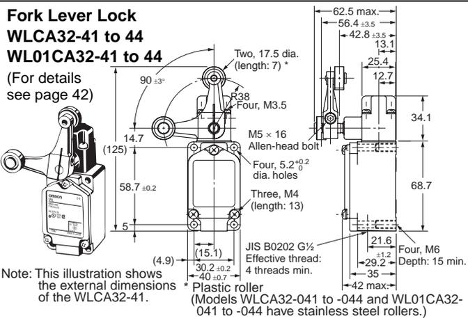
Note: This illustration shows the external dimensions of the WLCA32-41.
