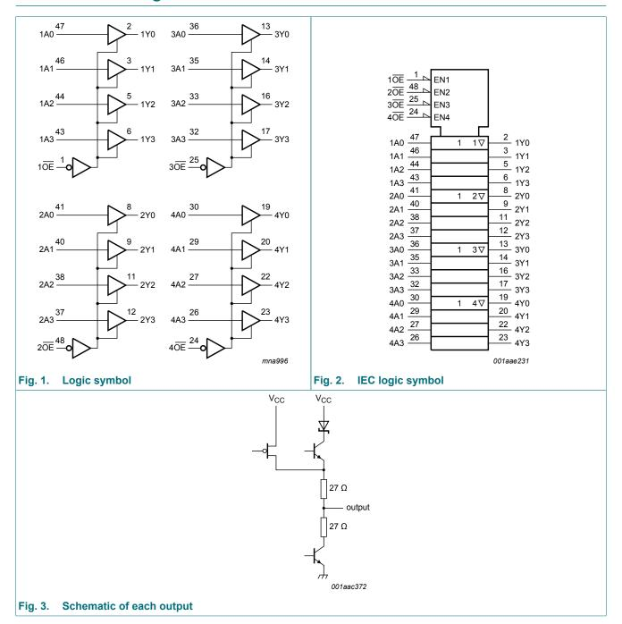
3.3 V 16-bit buffer/driver with 30  $\Omega$  termination resistors; 3-state
