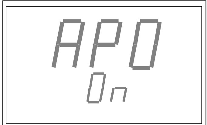
Figure 4. Automatic Power Off (APO) display
