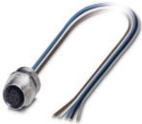
Sensor/actuator flush-type socket, 5-pos., M12, A-coded, front/screw mounting with Pg9 thread, with 4 m TPE litz wire, 5 x 0.34 mm 2
