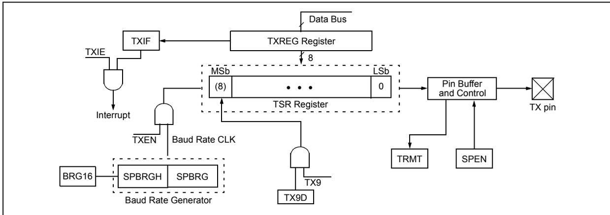
**FIGURE 18-4: ASYNCHRONOUS TRANSMISSION**
