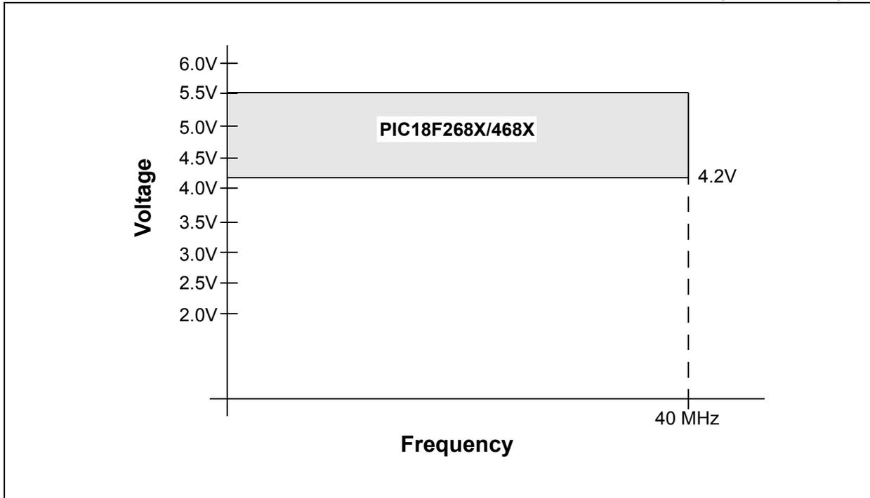
FIGURE 27-2: PIC18LF2682/2685/4682/4685 VOLTAGE-FREQUENCY GRAPH (INDUSTRIAL)
