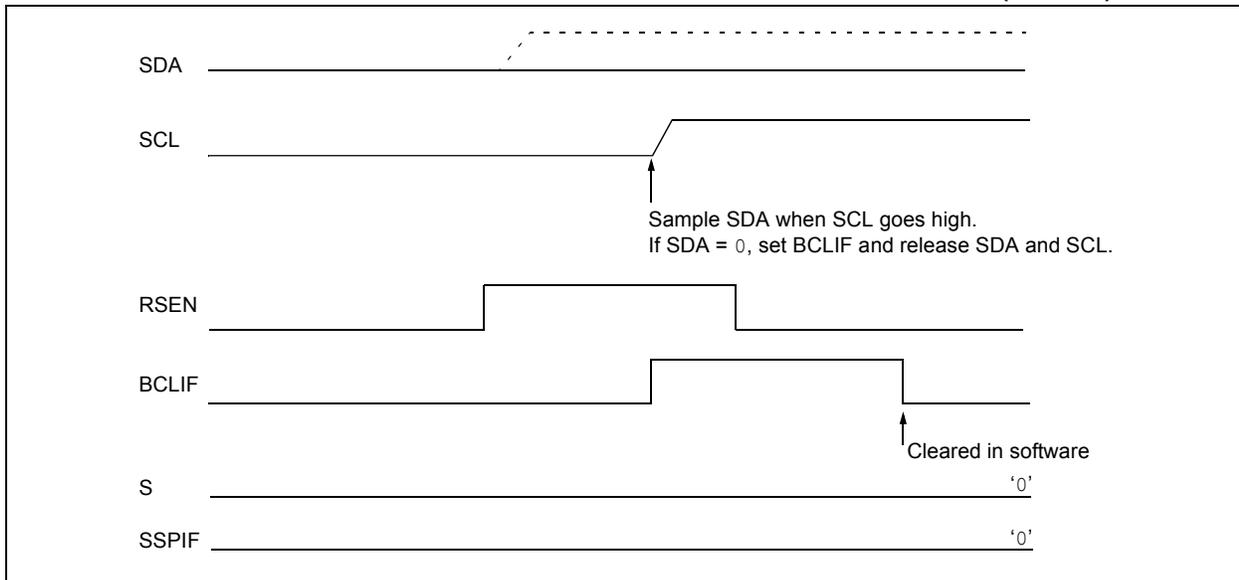
**FIGURE 17-30: BUS COLLISION DURING A REPEATED START CONDITION (CASE 2)**
