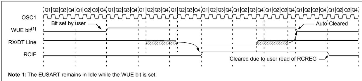
**FIGURE 18-9: AUTO-WAKE-UP BIT (WUE) TIMINGS DURING SLEEP**
