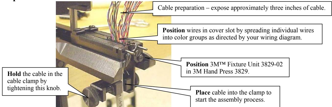
**Place** wires over and through cover slots and into slots of 3M™ Fixture Unit 3829-03 with a pulling-down motion to hold wire in place.
