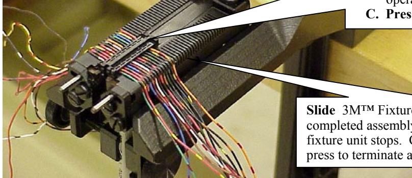
**Slide** 3M™ Fixture Unit 3829-02, with the completed assembly, into the hand press until the fixture unit stops. Close the handles of the hand press to terminate and trim the wires.
