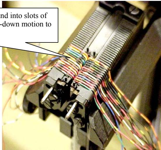
**Install** 3M™ Cutting Unit 3829-05. Push it in until it stops.
