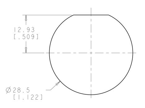
RECOMMENDED PANEL CUT-OUT MAX PANEL THICKNESS 3.2mm
