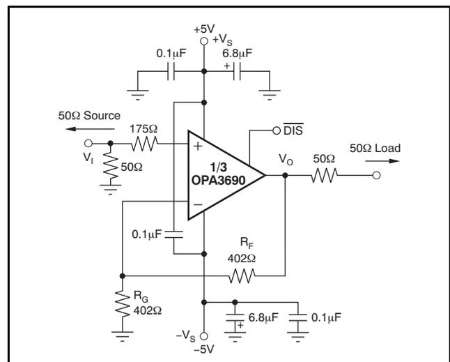
**Figure 36. DC-Coupled, G = +2, Bipolar-Supply Specification and Test Circuit**
