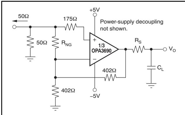
**Figure 48. Capacitive Load Driving with Noise Gain Tuning**
