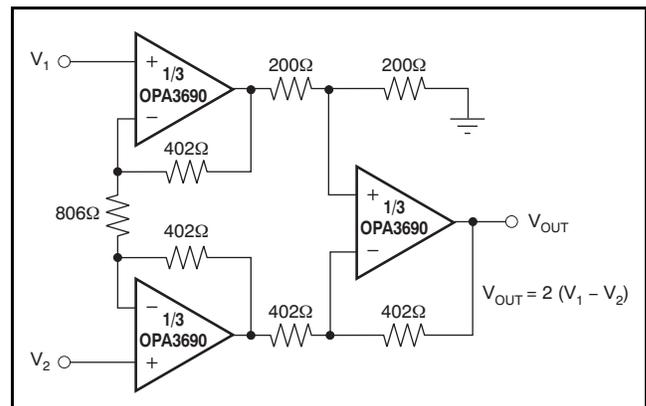
**Figure 41. Instrumentation Amplifier**
