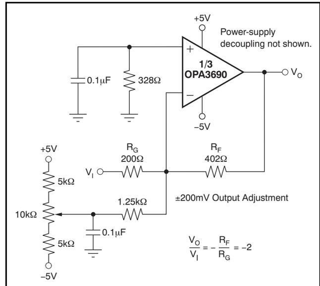
**Figure 51. DC-Coupled, Inverting Gain of –2, with Offset Adjustment**
