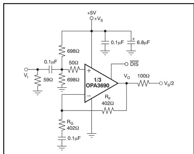
**Figure 37. AC-Coupled, G = +2, Single-Supply Specification and Test Circuit**
