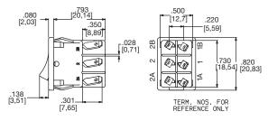
Actuator shown in pos. 1 – 'ON' position. SPST MODELS (D M14 & DM54) OMIT TERM INALS 2 & 2A.
