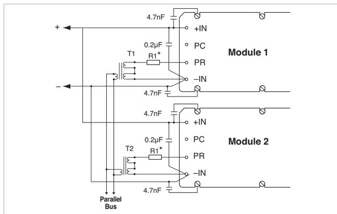
Figure 10 — Transformer-coupled interface
