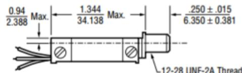
Model 78SBW (Adapter Pre-Assembled with Trimmer)
