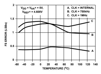
FIGURE 10. FULL SCALE ERROR vs TEMPERATURE
