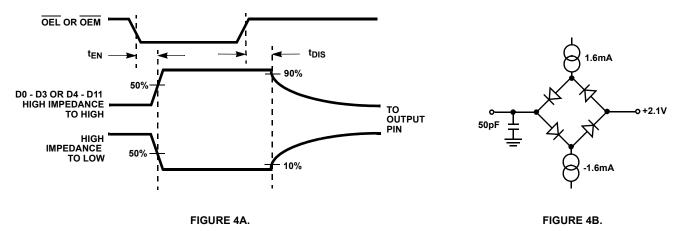
FIGURE 4. OUTPUT ENABLE/DISABLE TIMING DIAGRAM
