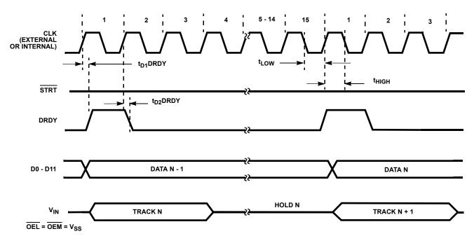
FIGURE 1. CONTINUOUS CONVERSION MODE
