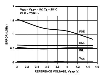
FIGURE 9. ACCURACY vs REFERENCE VOLTAGE
