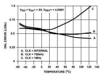
FIGURE 8. DNL vs TEMPERATURE
