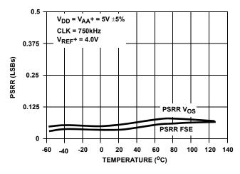
FIGURE 11. POWER SUPPLY REJECTION vs TEMPERATURE
