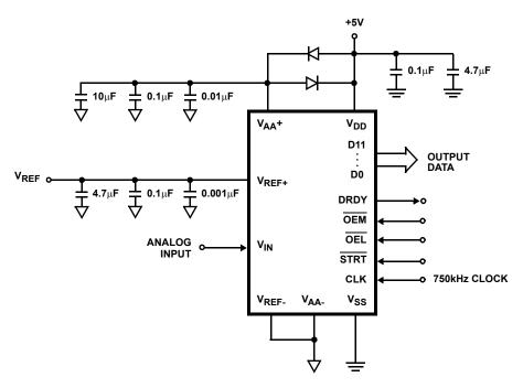
FIGURE 22. GROUND AND SUPPLY DECOUPLING
