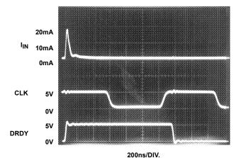
CONDITIONS:  $V_{DD} = V_{AA} + = 5.0V$ ,  $V_{REF} + = 4.608V$ ,  $V_{IN} = 4.608V$ , CLK = 750kHz,  $T_A = 25^{\circ}C$
