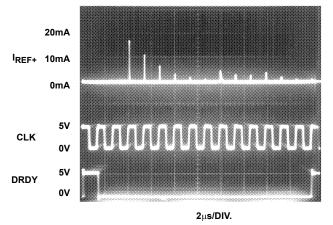
$\begin{aligned} \text{CONDITIONS:} \ \ V_{DD} = V_{AA} + = 5.0 \text{V}, \ V_{REF} + = 4.608 \text{V}, \\ V_{IN} = 2.3 \text{V}, \ CLK = 750 \text{kHz}, \ T_A = 25^{\text{O}} \text{C} \end{aligned}$
