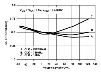
FIGURE 6. INL vs TEMPERATURE
