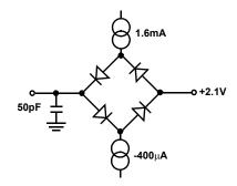
FIGURE 5. GENERAL TIMING LOAD CIRCUIT
