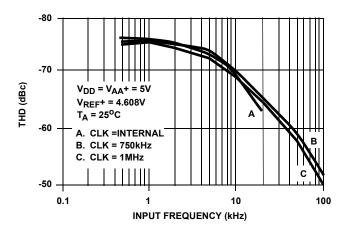
FIGURE 16. TOTAL HARMONIC DISTORTION vs INPUT FREQUENCY
