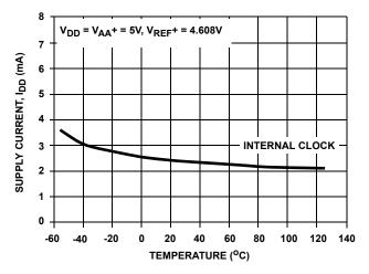
FIGURE 12. SUPPLY CURRENT vs TEMPERATURE
