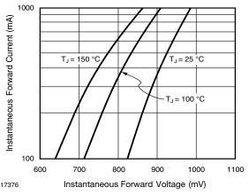
Fig. 2 - Typical Instantaneous Forward Characteristics
