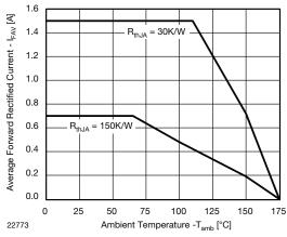
Fig. 1 - Forward Current Derating Curve
