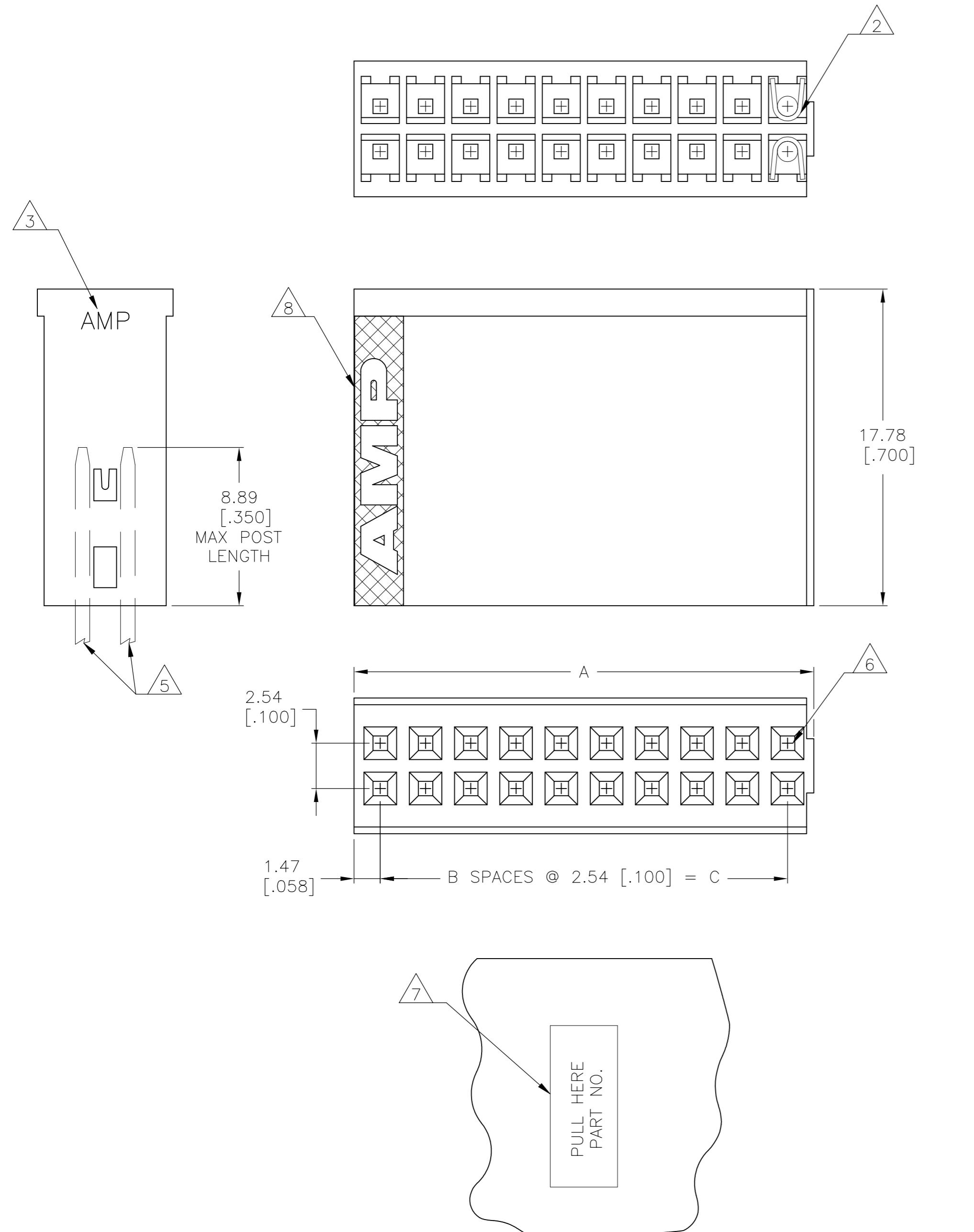
1 PULL ON HOUSING TO REMOVE FROM POSTS.
