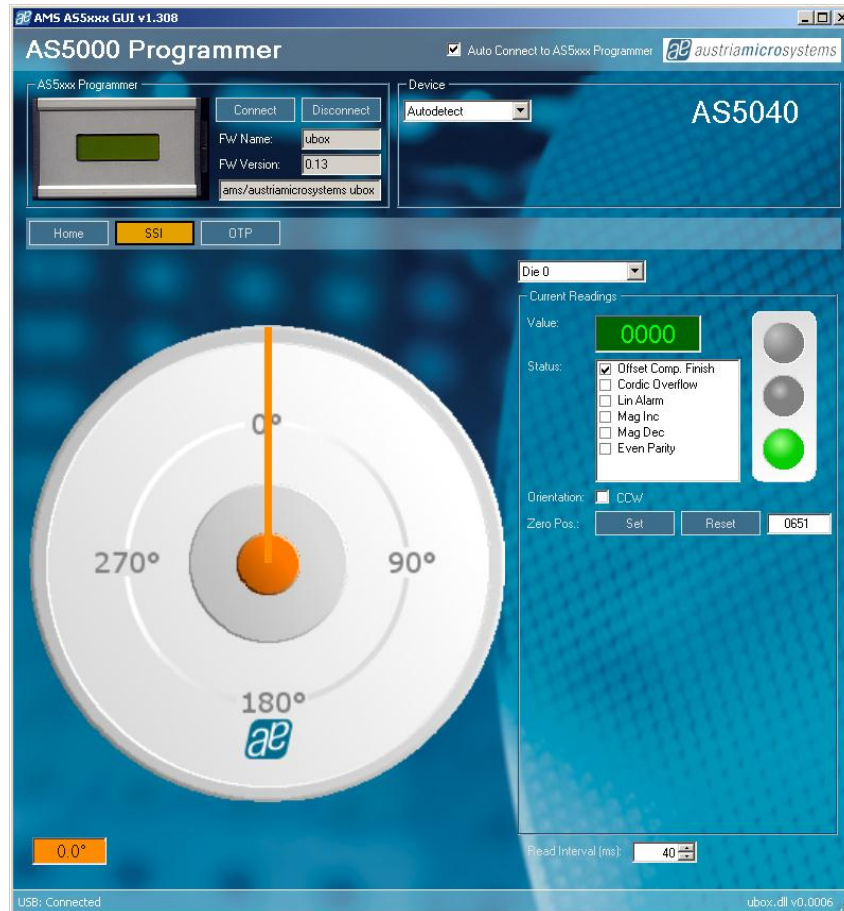
Figure 7: AS5040 SSI tab after Zero Position programming
