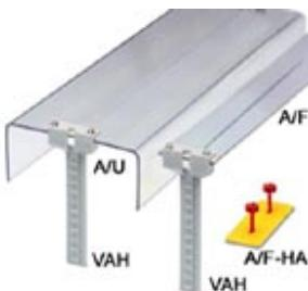
Flat-ribbon cover, for covering terminal strips, 2 mm thick, 7 cm wide, an additional requirement are 2 E/UK end brackets and 2 adjustable VAH cover holders. The max. supply length is 100 cm
