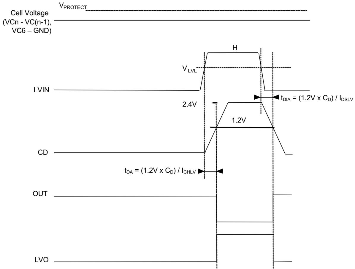
Figure 7. LVIN to OUT and LVO Timing
