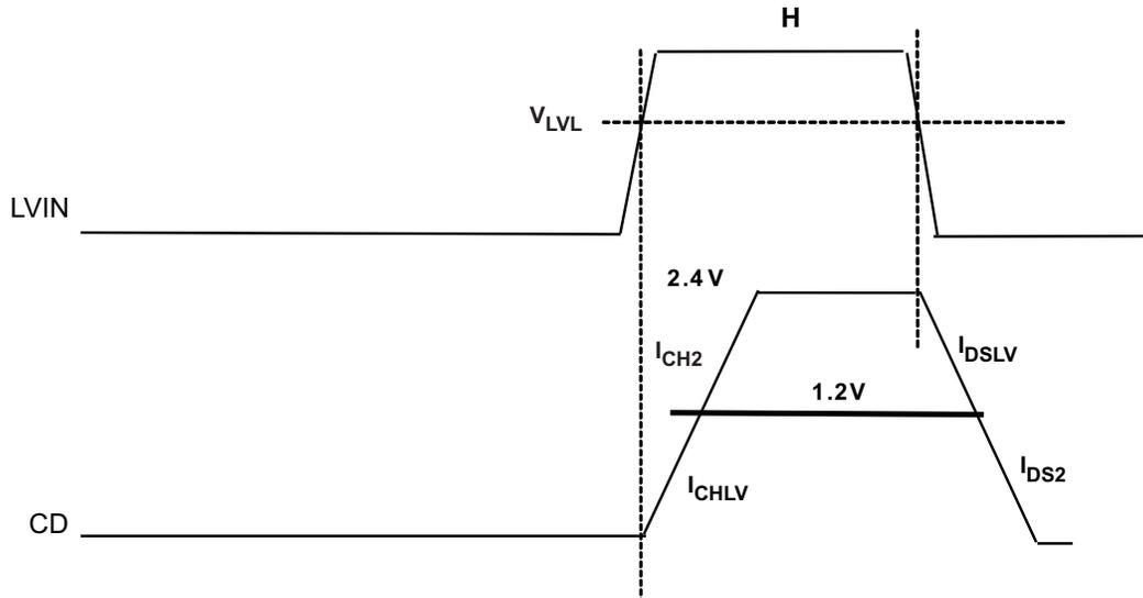
Figure 3. CD Charge Current and Discharge Current
