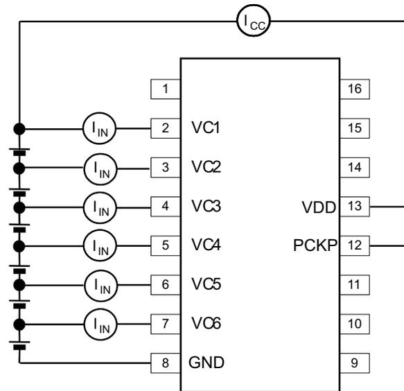
Figure 4.  $I_{CC}$ ,  $I_{IN}$  Measurement Test Setup
