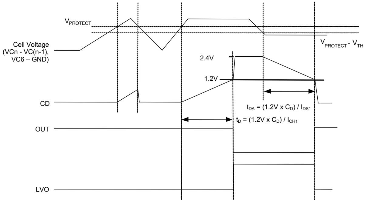
Figure 5. Timing for Overvoltage Sensing (With Recovery Option)
