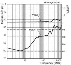
Note: High-frequency characteristics depend on the PCB to which the Relay is mounted. Always check these characteristics, including endurance, in the actual machine before use.
