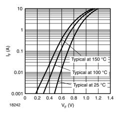
Fig. 1 - Typical Forward Characteristics
