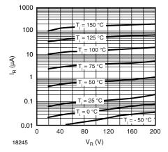
Fig. 4 - Typical Reverse Characteristics
