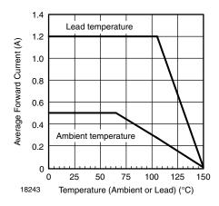
Fig. 2 - Forward Current Derating Curve
