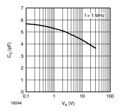
Fig. 3 - Typical Diode Capacitance vs. Reverse Voltage
