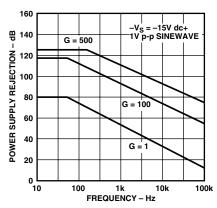
Figure 12. Positive PSRR vs. Frequency
