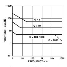
Figure 14. RTI Noise Spectral Density vs. Gain
