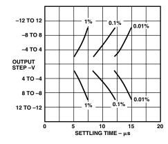
Figure 23. Settling Time Gain = 1000
