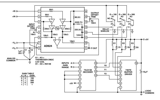
Figure 38. Gain Programmable Amplifier
