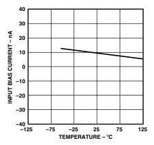
Figure 6. Input Bias Current vs. Temperature
