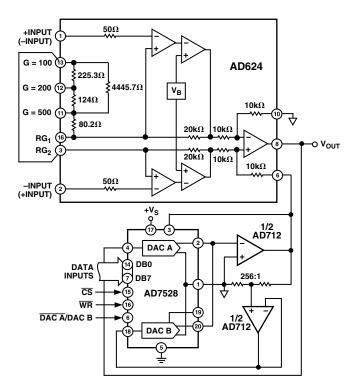
Figure 40. Programmable Output Gain Using a DAC
