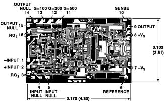
PAD NUMBERS CORRESPOND TO PIN NUMBERS FOR THE D-16 16-LEAD CERAMIC PACKAGE
