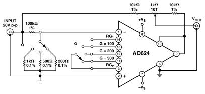
Figure 25. Settling Time Test Circuit
