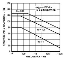
Figure 13. Negative PSRR vs. Frequency
