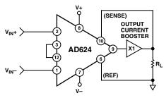
Figure 35. AD624 Instrumentation Amplifier with Output Current Booster
