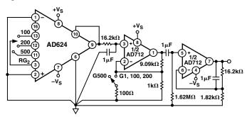
Figure 26. Noise Test Circuit
