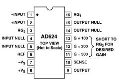
FOR GAINS OF 1000 SHORT  $\mathrm{RG}_1$  TO PIN 12 AND PINS 11 AND 13 TO  $\mathrm{RG}_2$
