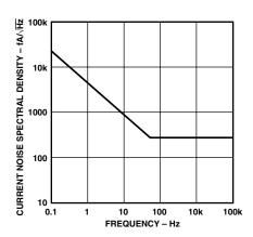
Figure 15. Input Current Noise
