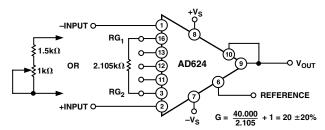
Figure 29. Operating Connections for G = 20
