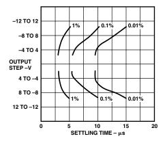
Figure 18. Settling Time, Gain = 1
