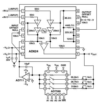
Figure 39. Programmable Output Gain
