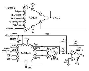
Figure 41. Software Controllable Offset
