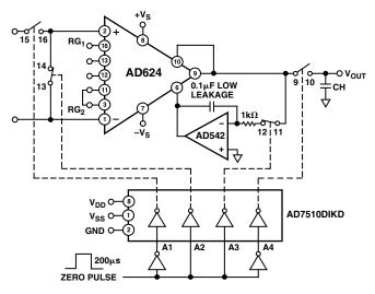
Figure 42. Autozero Circuit
