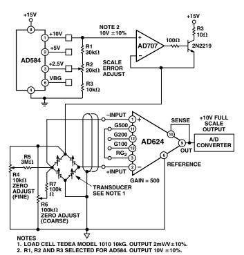
Figure 44. AD624 Weigh Scale Application
