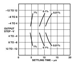
Figure 20. Settling Time Gain = 100
