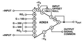
Figure 28. Operating Connections for G = 200
