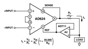
Figure 37. Voltage-to-Current Converter
