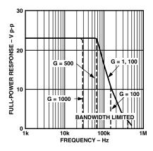
Figure 11. Large Signal Frequency Response
