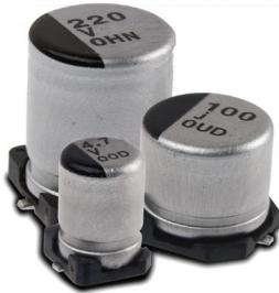
Type AVES Capacitors are rated for 1000 hours at  $105^{\circ}\text{C}$  with low impedance characteristics. They are ideal for high density PC board packaging. The Type AVES offers a low in-place-cost for a high quality performer. The vertical cylindrical cases facilitate automatic mounting and reflow soldering into the same footprint of like-rated tantalum capacitors except without the need for voltage derating.
