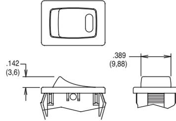
**NOTE:** Available with DA102 switch function and 6 lamp rating combinations only. Not available with O2 and A termination options. \* J5 actuator not available with Termination option "17" solder lug
