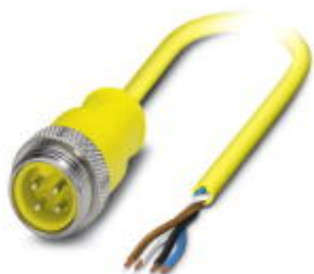
Sensor/actuator cable, 4-position, PVC, yellow, Plug straight 7/8"-16UNF, A-coded, on free cable end, cable length: 2 m
