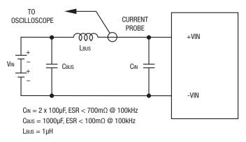
Figure 4: Measuring Input Ripple Current
