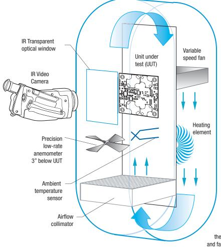
Figure 9. Vertical Wind Tunnel
