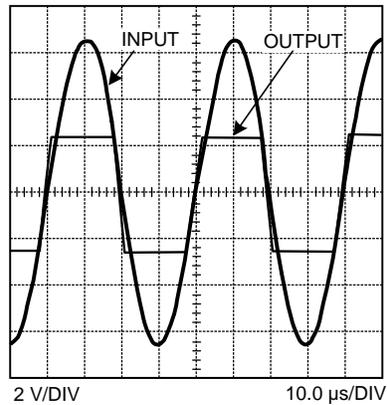
**Figure 45. Input/Output Shown with Exceeded Input CMVR**
