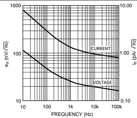
Figure 8. Noise vs. Frequency
