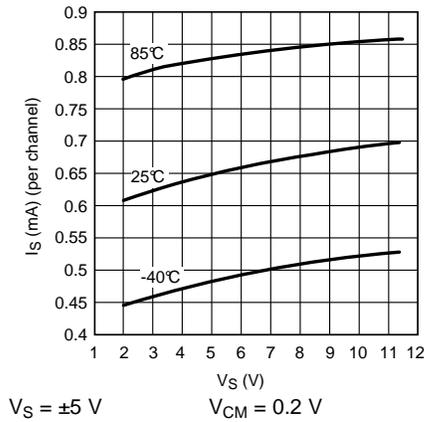
Figure 33.  $I_S$  (mA) vs.  $V_S$ (V)
