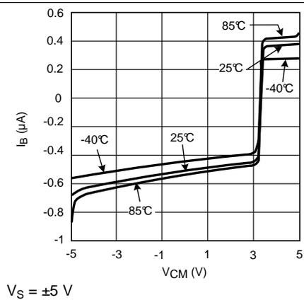
Figure 30.  $I_B$  vs.  $V_{CM}$
