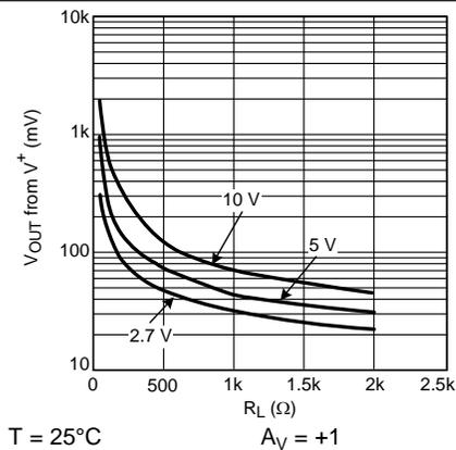
Figure 11. Output Swing from  $V^+$  vs.  $R_L$  (tied to  $V_S/2$ )
