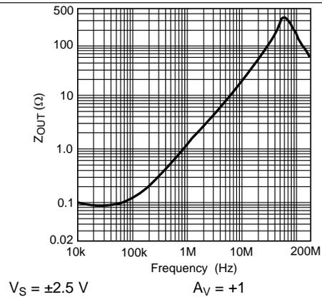
Figure 18.  $Z_{OUT}$  vs. Frequency
