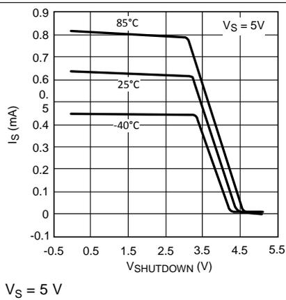
Figure 35.  $I_S$  vs.  $V_{SHUTDOWN}$  (LMH6647)
