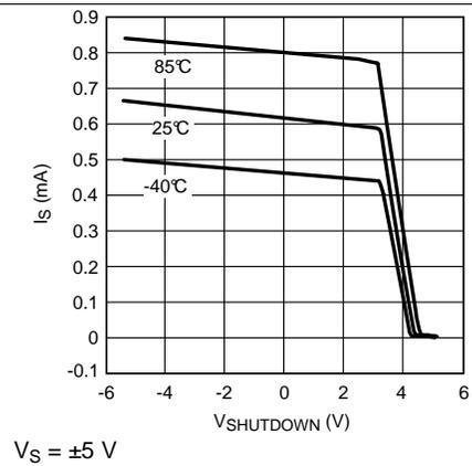
Figure 36.  $I_S$  vs.  $V_{SHUTDOWN}$  (LMH6647)
