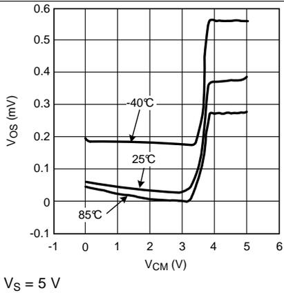
Figure 27.  $V_{OS}$  vs.  $V_{CM}$  (a Typical Unit)
