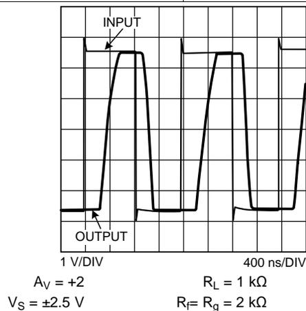
Figure 41. Output Overload Recovery
