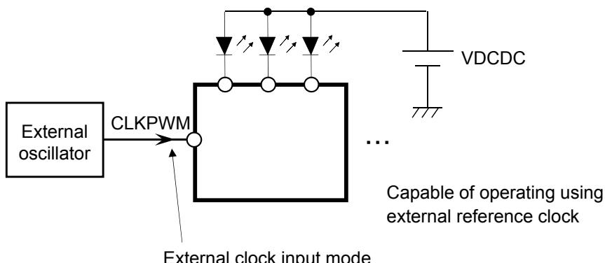
Capable of operating using external reference clock
