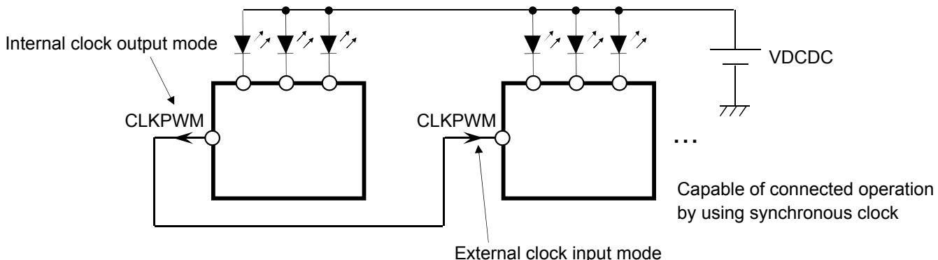
Capable of connected operation by using synchronous clock
