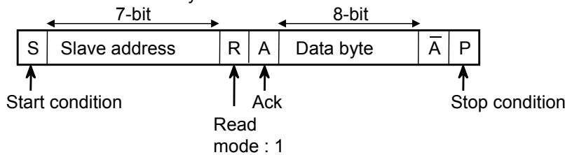
Ex) When writing data into address and reading data from "01 h"
