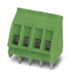
PCB terminal block, Nominal current: 24 A, Nom. voltage: 400 V, Pitch: 5.08 mm, Number of positions: 4, Connection method: Screw connection with tension sleeve, Mounting: Wave soldering, Conductor/PCB connection direction: 55 °, Color: green, The article can be aligned to create different nos. of positions!
