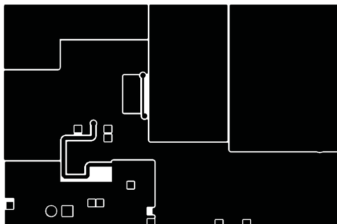
Figure 44. TPS40200EVM-001 Bottom Copper (X-Ray View From Top)
