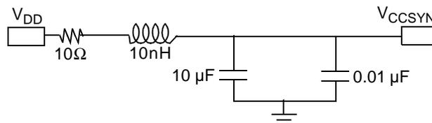
**Figure 34.  $V_{CCSYN}$  Bypass**
