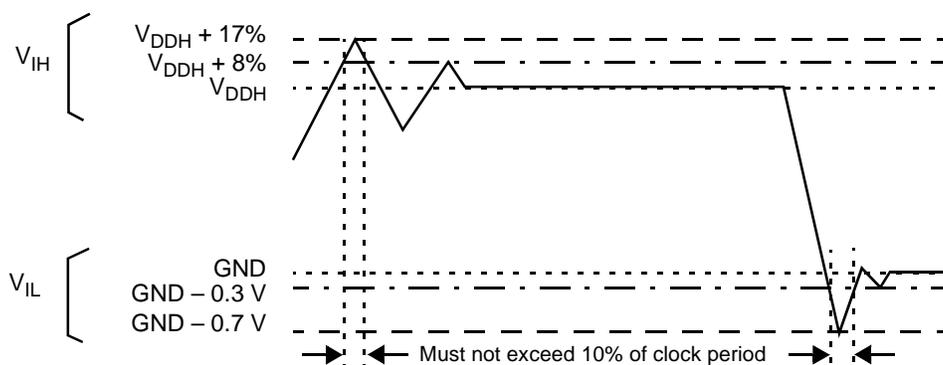
Figure 5. Overshoot/Undershoot Voltage for  $V_{IH}$  and  $V_{IL}$
