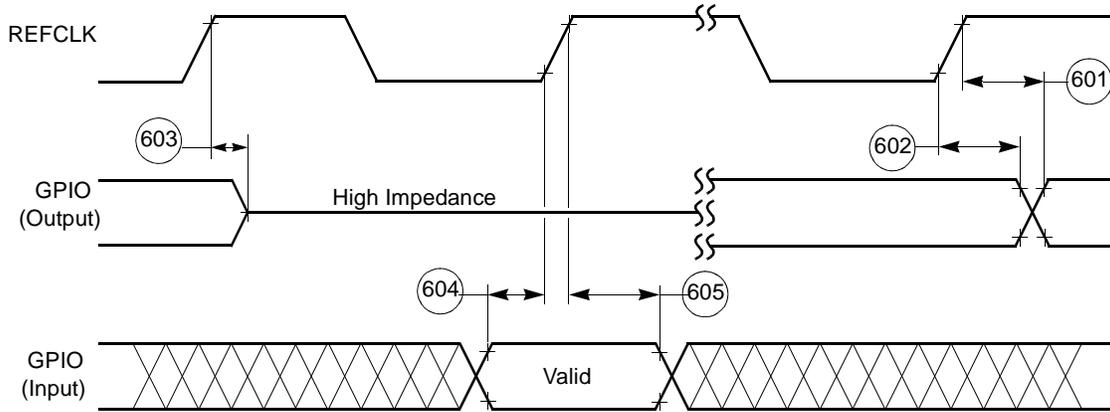
Figure 27. GPIO Timing
