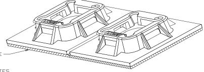
ADHESIVE BACKING: (-A , -AT) RUBBER OR ACRYLIC BASED ADHESIVE PRESSURE SENSITIVE FOAM TAPE 0.04 [1.0] THICK WITH A PROTECTIVE LINER, MOUNT IS DESIGNED TO SUPPORT 0.50 16s (227g) MAX. WEIGHT ON A CLEAN DRY SMOOTH SURFACE.
