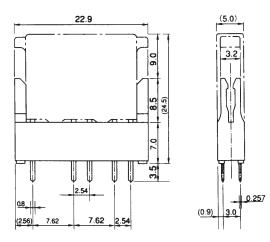
Note: Tolerance for PC board mounting hole/pad layout: +/-0.1. Note: Dimensions of the terminals do not include thickness of pre-solder. Note: This datasheet provide only + tolerance for outer dimensions. Please ask for specification in case you need other tolerances.
