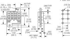
PC board layout for 4 pole PCB terminal socket
