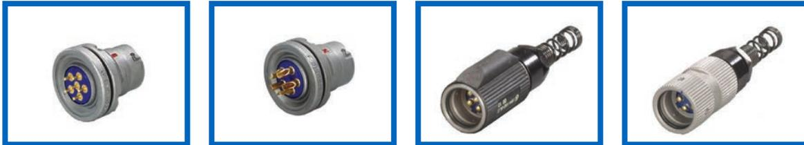
**MW Series Power Connectors** are qualified to MIL-DTL-55181. They are designed with a center lock coupling screw. The connectors are waterproof, polarized and can withstand high shock and vibrations. They are primarily used for interconnection of power and control circuits of electric equipment by the US Army Communication System.
