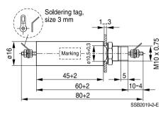
Tightening torque: 3 +0.5 Nm General tolerances according to ISO 2768-cL Dimensions in mm
