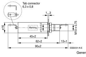
31-K-E Tightening torque: 3 +0.5 Nm General tolerances according to ISO 2768-cL Dimensions in mm
