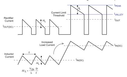
Figure 19. Inductor/Rectifier Currents in Current Limit Operation (DC/DC Boost Mode)
