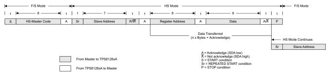
Figure 26. Data Transfer Format in H/S-Mode
