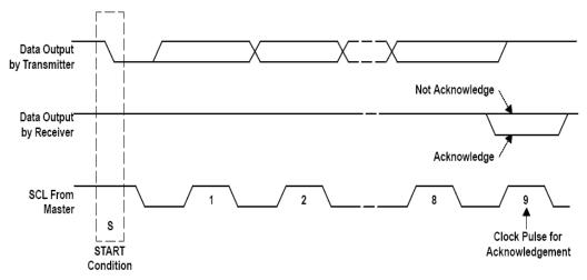
Figure 22. Acknowledge on the I<sup>2</sup>C Bus
