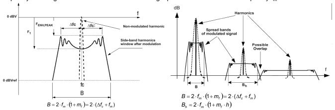
Figure 15. Spectrum of a Frequency Modulated Sin. Wave with Sinusoidal Variation in Time
