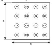
Figure 66. CHIP SCALE PACKAGE (BOTTOM VIEW)
