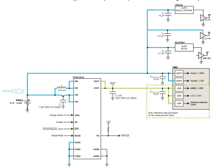
Figure 28. TPS61281A Application Circuit with 1500mA Output Current
