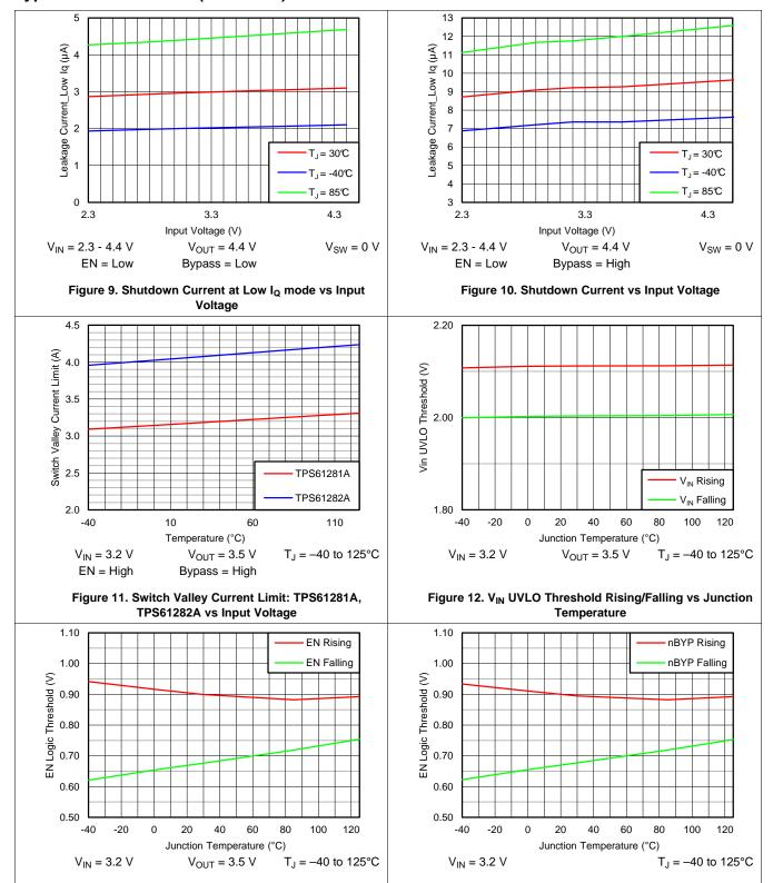
Figure 13. EN Logic High Threshold Rising/Falling vs
