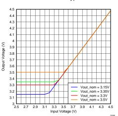
Figure 18. DC Output Voltage vs. Input Voltage
