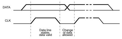
Figure 21. Bit Transfer on the Serial Interface
