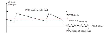
Figure 17. Power-Save Mode Ripple
