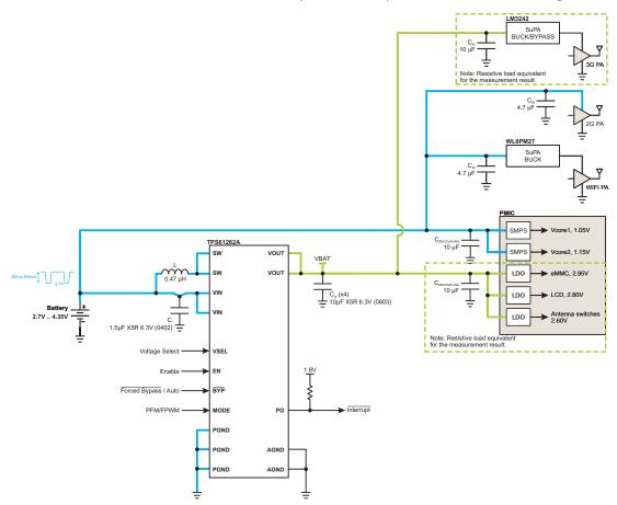
Figure 48. TPS61282A Application Circuit with 2000 mA Output Current
