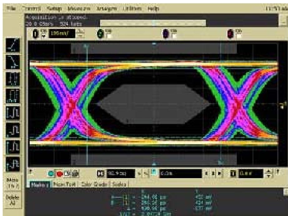
Figure 6: 8bit deep color DVI/HDMI TX eye tested with 25 meter. 24 AWG HDMI cable. Setting: Optimized equalization, 0dB output pre-emphasis and de-emphasis, and Swing 500mV.
