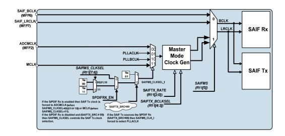
Figure 31 SAIF Interface Clock Configuration
