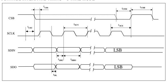
Figure 4 SPI Compatible Control Interface Input Timing
