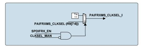
Figure 36 Manual Clock Over-ride of PAIF Rx
