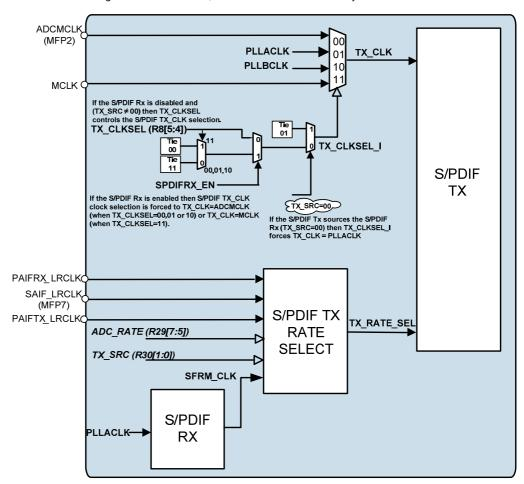
Figure 28 S/PDIF TX Clock and Rate Selection
