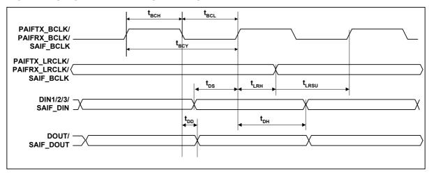
Figure 3 Digital Audio Data Timing - Slave Mode
