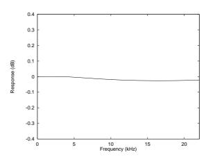
Figure 47 De-Emphasis Frequency Response (44.1kHz)
