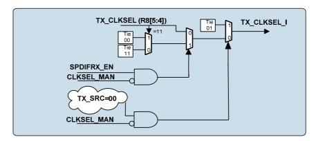
Figure 34 Manual Clock Over-ride of S/PDIF Tx Clock
