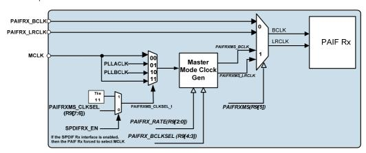
Figure 29 PAIF Rx Interface Clock Configuration
