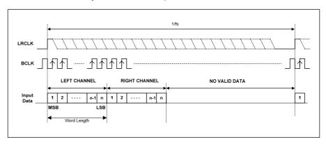
Figure 21 DSP Mode B Timing Diagram - SAIF Receiver Input Data
