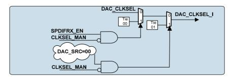
Figure 32 Manual Clock Over-ride of DAC Clock
