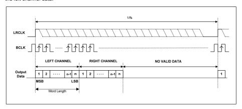
Figure 22 DSP Mode B Timing Diagram - PAIF/SAIF Transmitter Data
