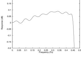
Figure 44 DAC Digital Filter Ripple -44.1, 48 and 96kHz
