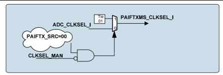
Figure 35 Manual Clock Over-ride of PAIF Tx
