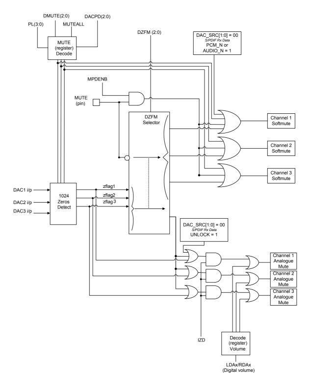
Figure 24 Mute Mode Block Diagram
