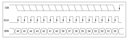
Figure 6 3-Wire SPI Compatible Interface
