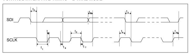
Figure 5 Control Interface Timing – 2-Wire Serial Control Mode
