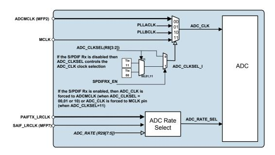
Figure 27 ADC Clock and ADC Rate Selection
