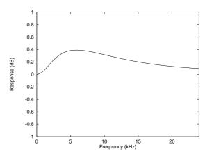
Figure 49 De-Emphasis Frequency Response (48kHz)
