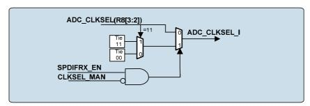
Figure 33 Manual Clock Over-ride of ADC Clock
