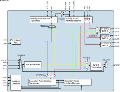
Figure 25 Digital Routing
