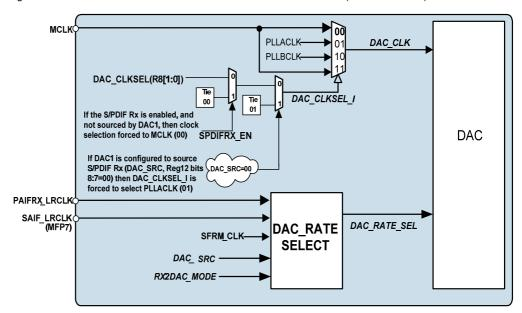
Figure 26 DAC Clock and DAC Rate Selection
