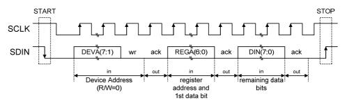
Figure 9 2-Wire Serial Control Interface
