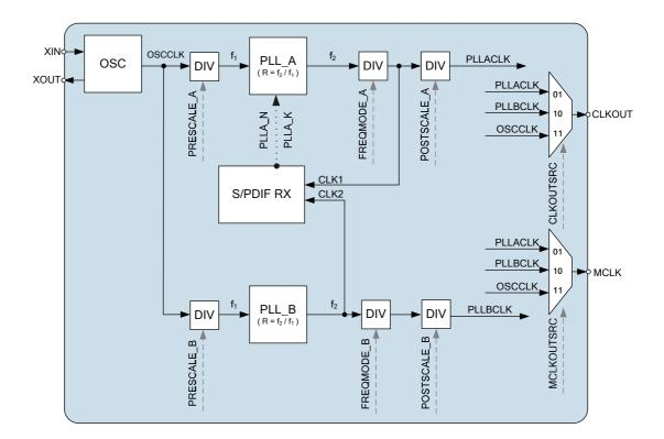
Figure 38 PLL and Clock Select Circuit
