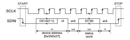
Figure 10 2-Wire Continuous Readback
