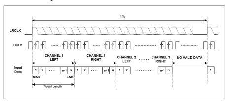
Figure 20 DSP Mode B Timing Diagram - PAIF Receiver Input Data
