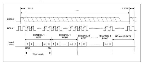
Figure 17 DSP Mode A Timing Diagram - PAIF Receiver Input Data
