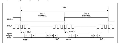
Figure 16 I<sup>2</sup>S Mode Timing Diagram
