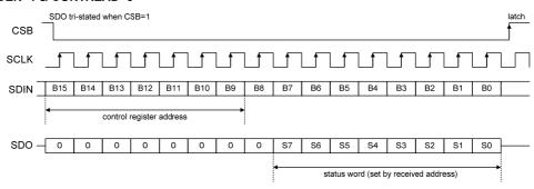
Figure 8 3-Wire SPI Compatible Control Interface Non-Continuous Readback
