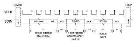
Figure 11 2-Wire Non-Continuous Readback
