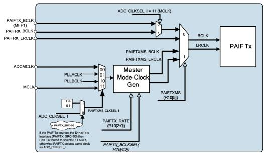
Figure 30 PAIF Tx Interface Clock Configuration
