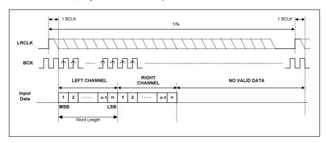
Figure 18 DSP Mode A Timing Diagram – SAIF Receiver Input Data
