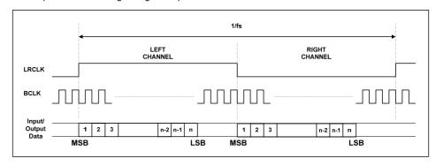
Figure 14 Left Justified Mode Timing Diagram
