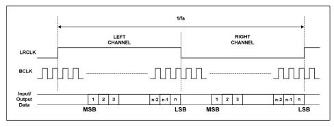
Figure 15 Right Justified Mode Timing Diagram
