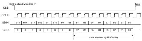
Figure 7 3-Wire SPI Compatible Interface Continuous Readback
