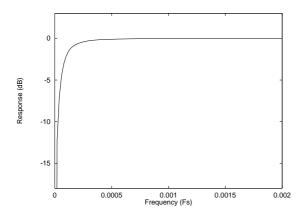
Figure 53 ADC Highpass Filter Response
