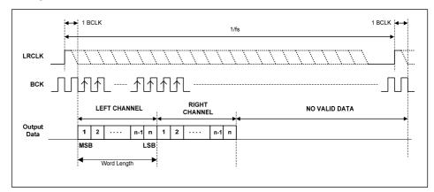
Figure 19 DSP Mode A Timing Diagram - PAIF/SAIF Transmitter Data
