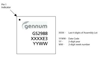
Figure 6-4: Marking Diagram
