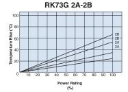
PCB: FR-4t = 1.6mm Cu foil thickness: 35µm ①: Hot spot
