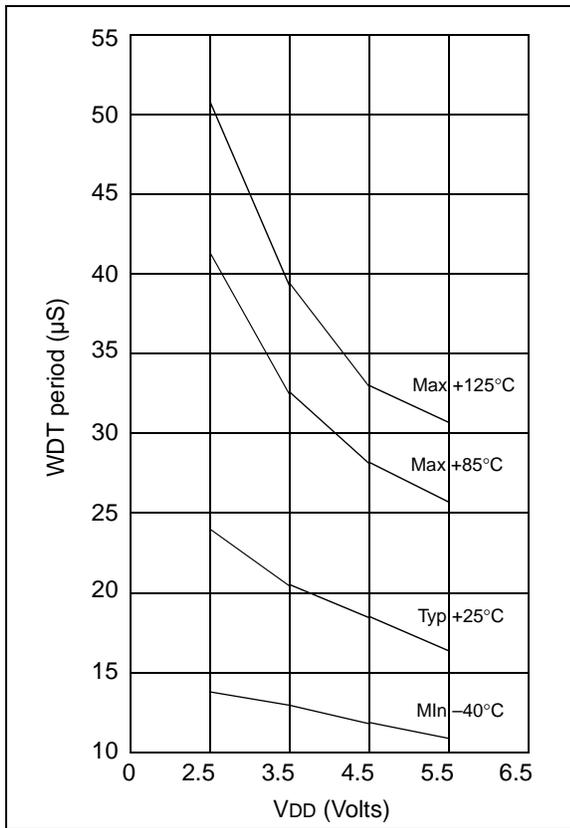
**FIGURE 11-4: SHORT DRT PERIOD VS. V<sub>DD</sub>**
