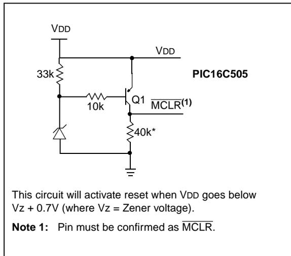
**FIGURE 7-13: BROWN-OUT PROTECTION CIRCUIT 2**
