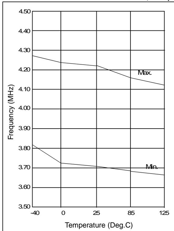
**FIGURE 11-2: CALIBRATED INTERNAL RC FREQUENCY RANGE VS. TEMPERATURE (V<sub>DD</sub> = 2.5V) (INTERNAL RC IS CALIBRATED TO 25°C, 5.0V)**
