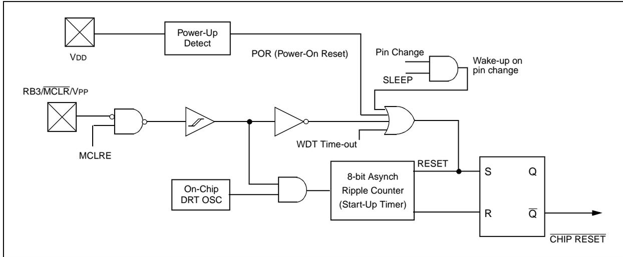
**FIGURE 7-8: TIME-OUT SEQUENCE ON POWER-UP ( $\overline{\text{MCLR}}$  PULLED LOW)**
