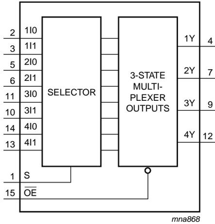
Fig 3. Functional diagram
