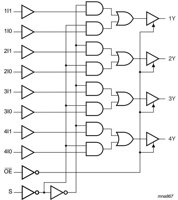
Fig 4. Logic diagram
