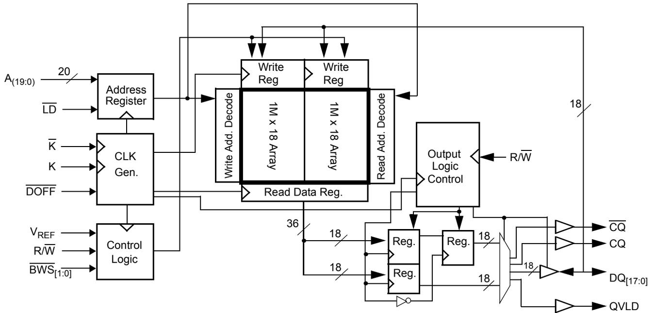
Logic Block Diagram – CY7C1270KV18
