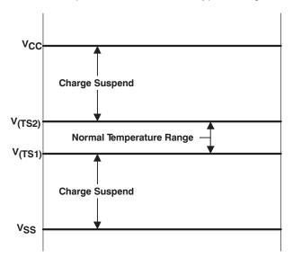
Figure 6. TS Pin Thresholds
