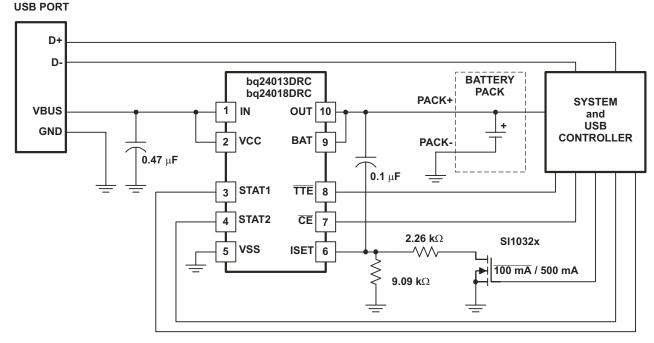
Figure 4. USB Charger Circuit
