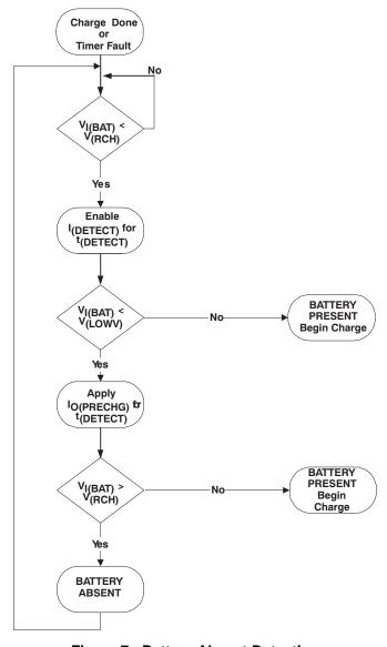
Figure 7. Battery Absent Detection
