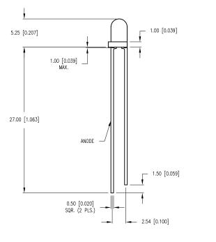
\*UNLESS OTHERWISE SPECIFIED TOLERANCES PER DECIMAL PRECISION ARE: X=±1 (±0.039), XX=±0.5 (±0.020), XXX=±0.25 (±0.010), XXXX=±0.127 (±0.005). LEAD SIZE=±0.05 (±0.002), LEAD LENGTH=±0.75 (±0.030). MIN=  $\frac{+0.00}{-0.00}$  MAX.=  $\frac{+0.00}{-0.00}$  MAX
