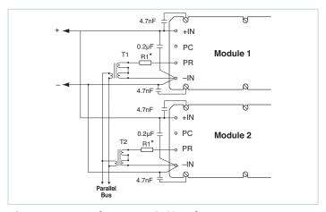
Figure 10 — Transformer-coupled interface
