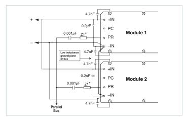
Figure 9 — AC coupled single-wire interface
