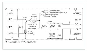
Figure 3 — PC/SC module alarm logic
