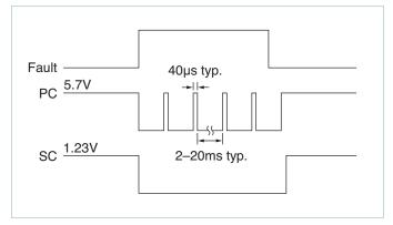
Figure 5 — PC/SC module alarm timing
