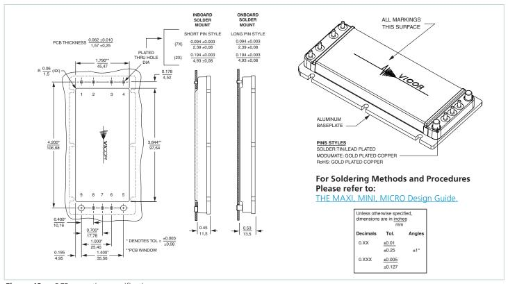
Figure 13 — PCB mounting specifications
