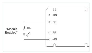
Figure 4 — LED on-state indicator
