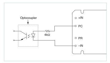
Figure 6 — Isolated on-state indicator
