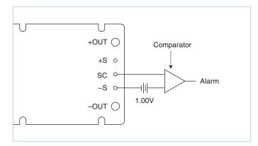
Figure 7 — Secondary side on-state indicator
