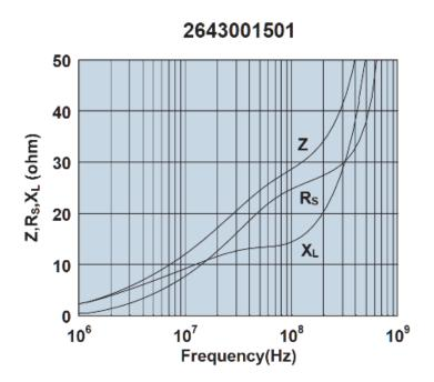
Impedance, reactance, and resistance vs. frequency.
